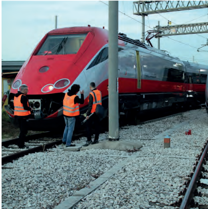
The two Frecciarossa high-speed trains are 328 metres long and can travel at speeds of up to 360 kilometres per hour. In their noses, the scientists installed measurement antennas and a proximity radar to accurately determine the distance between the two trains and exchange information between them.
