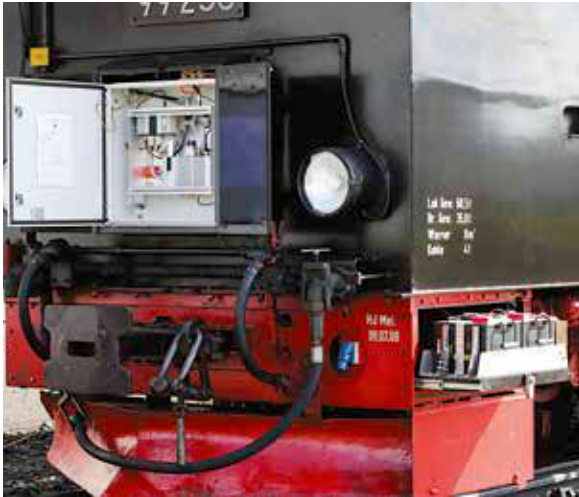
The TrainCAS onboard unit includes a Moxa processor and a driver advisory display, along with a separate battery pack.
